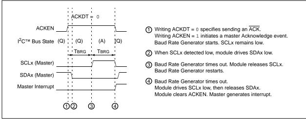
Figure 24-12: Master Not Acknowledge (NACK) Timing Diagram
