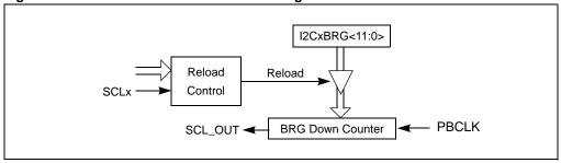
Figure 24-6: **Baud Rate Generator Timing with Clock Arbitration**
