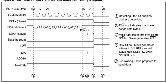
Figure 24-23: Slave Read 7-bit Address Detection Timing Diagram
