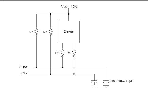
Note: I<sup>2</sup>C™ devices with input levels related to VDD must have one common supply line to which the
