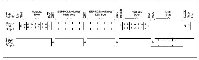
The I<sup>2</sup>C module supports Master mode communication with the inclusion of Start and Stop generators, data byte transmission, data byte reception, an Acknowledge generator and a BRG. Generally, the software will write to a control register to start a particular step, and then wait for an interrupt or poll status to wait for completion. Subsequent sections detail each of these operations.
